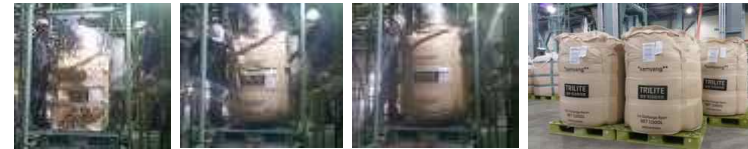
(Manual packing line : 1,000 ℓ Bag, plastic/fiber drum)
